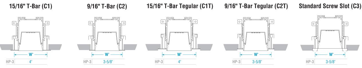
• NOTE: Only for standard 2x4 or 2x2 T-Bar ceiling, the starter luminaire is purposefully short by 1-1/8" to ensure fit in T-Bar types, shown above.
