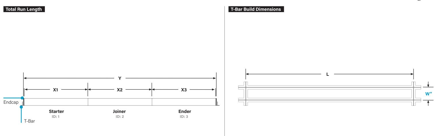
X = Luminaire section length (**Does not include endcaps**)
