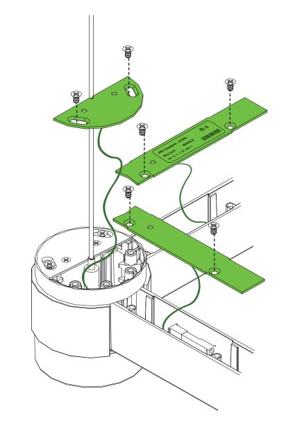
Replace all Cover Plate and turn power on to luminaire
