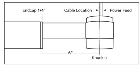
**NOTE:** Our Standard Configurations are available with a single 18/5 feed into 1 or 2 arm Knuckle. 3 and 4 arm Knuckles do not accept power feeds. Consult factory for available options regarding feeds, multiple circuits, and emergency wiring. Feed locations will be confirmed on the shop drawings.
