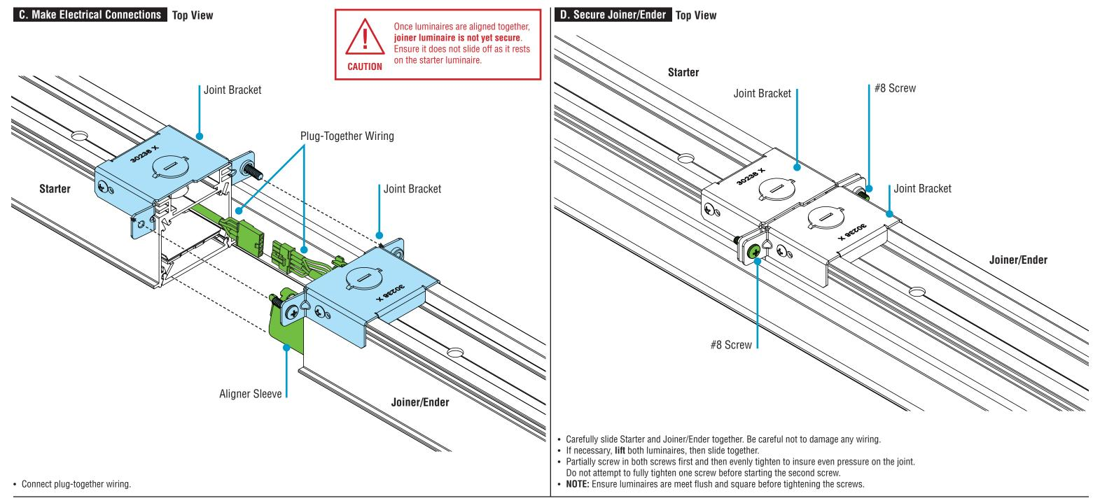
Simple Plug-Together Wiring
