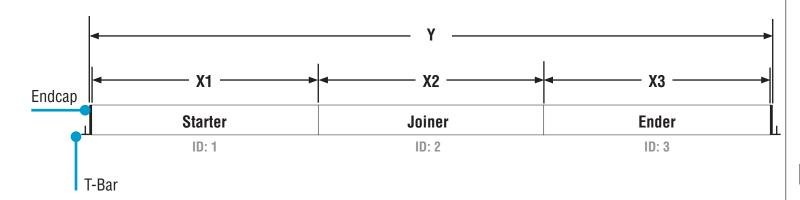
**X** = Luminaire section length (**Does not include** endcaps)
