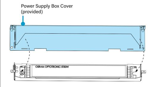
Rotate driver and cover back into position, carefully tuck in wires to avoid any pinched wires.
