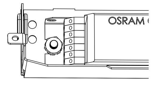
Tip driver out, and tip in new driver in the same orientation as old driver, hook in one end and then resecure driver using kep nut.
