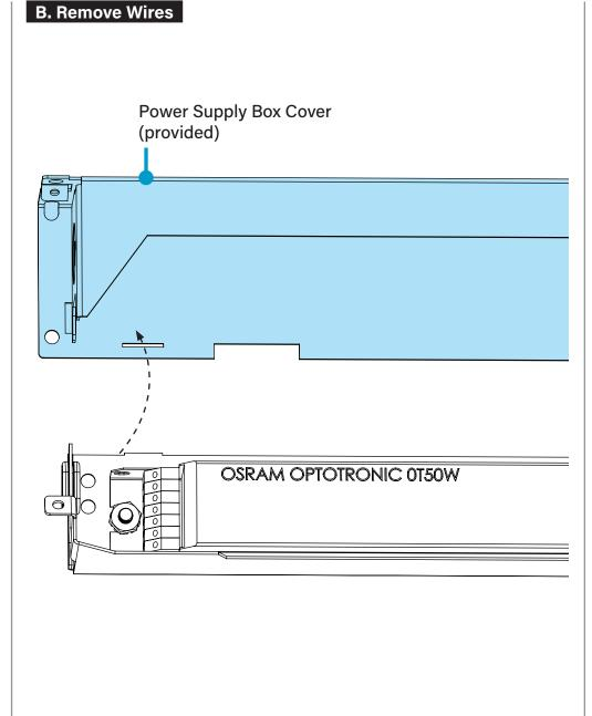
Remove wires from driver by depressing driver terminal block with tip of small slotted screw driver.
