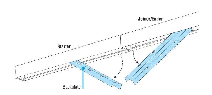
• Carefully rotate backplates out **at the joints only** and let them hang from luminaire body.
