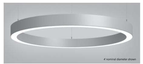
High Performance 2" Aperture Circle (HP-2 C) is a patented, circular LED luminaire. Constructed with an extruded aluminum body and single-piece direct diffuser, the HP-2 C provides a seamless finish aesthetic. Delivering excellent performance using an advanced optical design and mid-power LEDs to achieve 90% of initial light output at 100,000+ hours.
