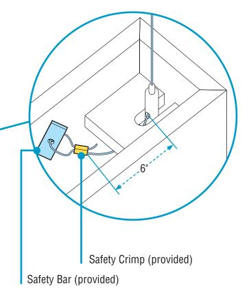
• Estimate required length of cable and add 8" • Loop cable through Safety Crimp and Safety Bar, then back through Safety Crimp. • Crimp, then cut excess cable. Remaining 6" of cable.
