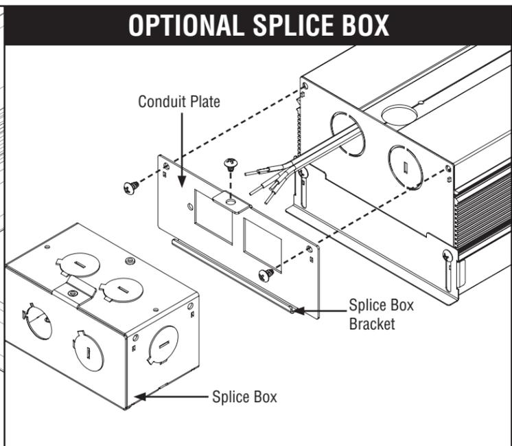
Attach optional splice box to conduit plate by hooking onto splice box bracket. Insert wires through feed hole.
