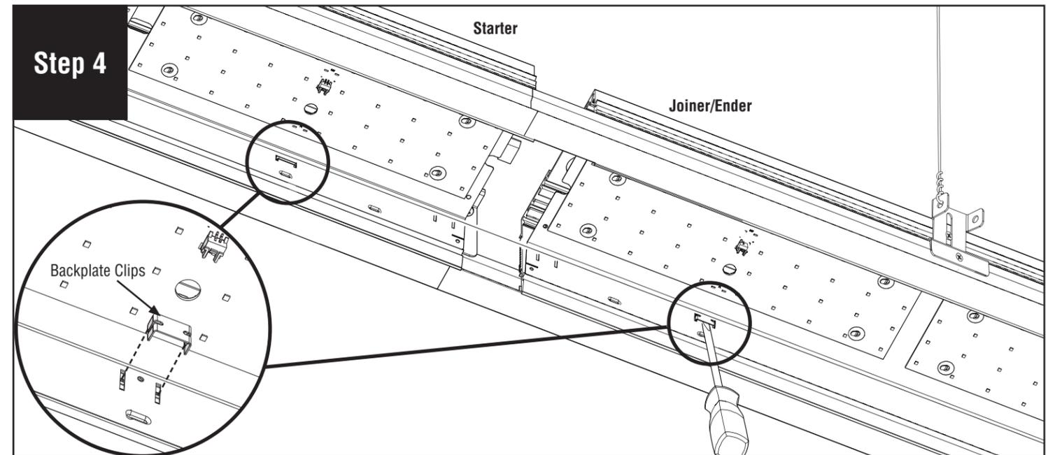
Remove backplate clips to release the backplate. We recommend using a flat head screwdriver to remove them. **CAUTION: Do not lose these pieces.**
