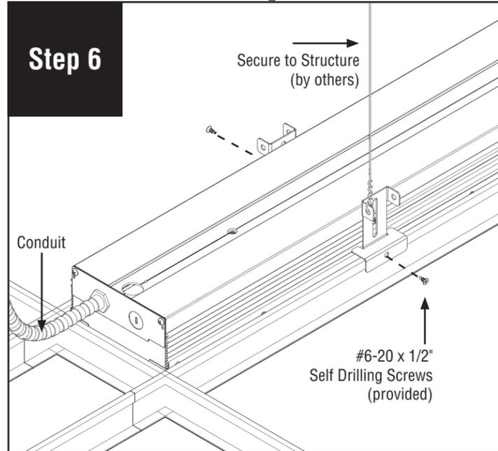
Secure luminaire to T-Bar with #6-20 x 1/2" self drilling sheet metal screws (provided).
