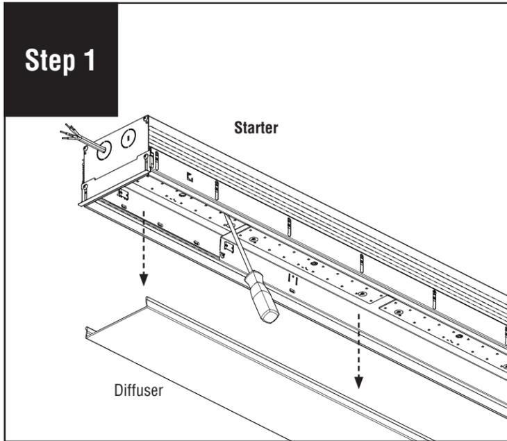
Remove diffuser and set aside to prevent it from getting dirty or damaged. **NOTE:** If part of a longer run, diffuser will be reinstalled back into original luminaire section as lengths vary.
