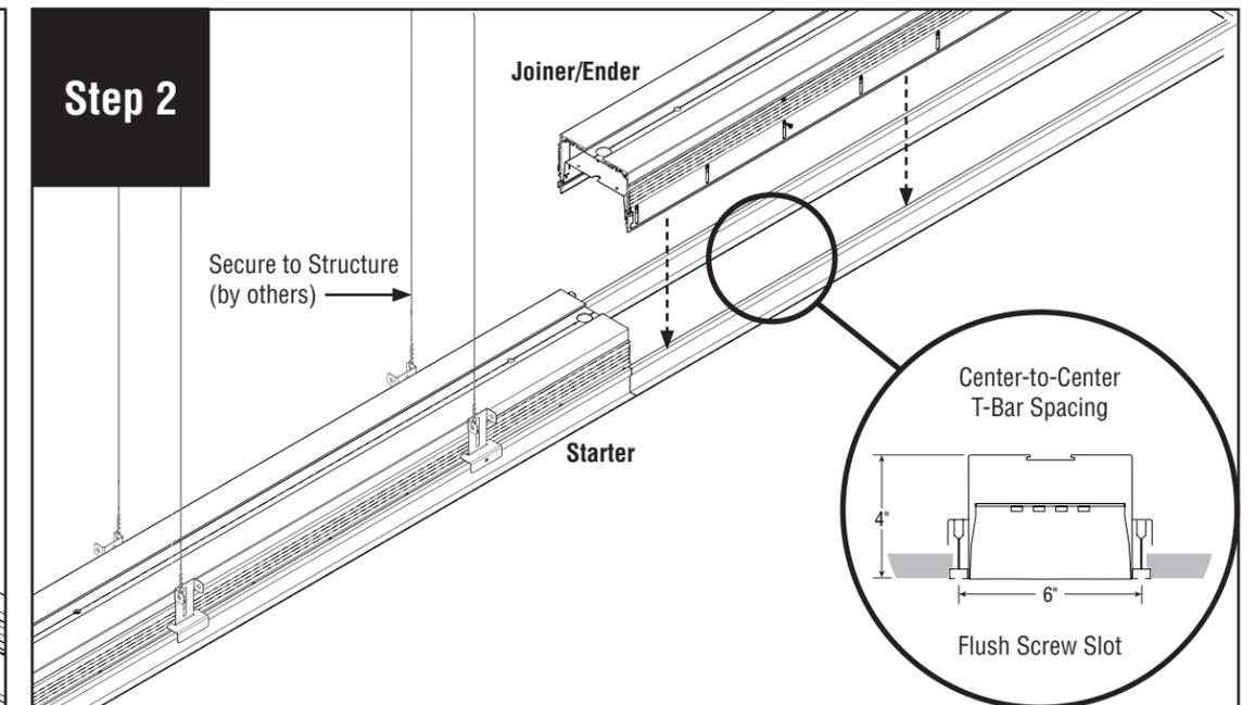
Install joiner/ender onto ceiling next to starter.
