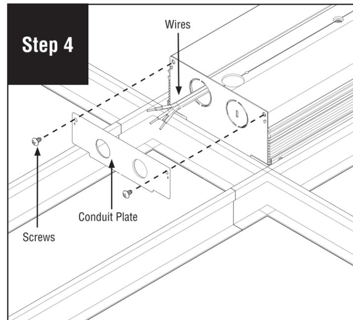
Remove conduit plate from luminaire. **NOTE:** Purple and gray wires are for Low Voltage Control.
