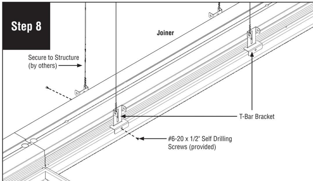
Secure luminaire to T-Bar with #6-20 x 1/2" self drilling sheet metal screw (provided).
