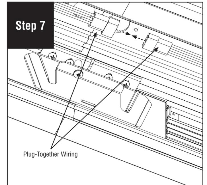
Connect plug-together wiring connections.
