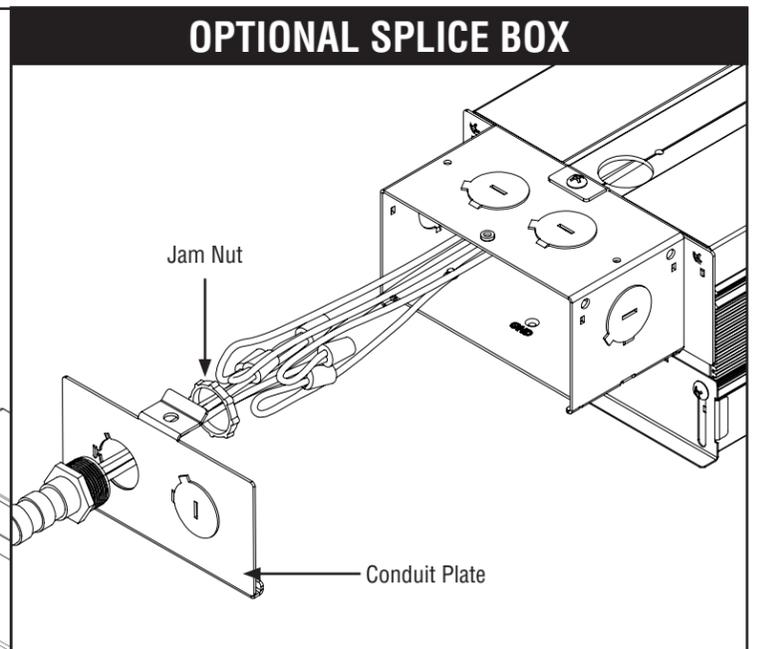
Run power cable through knock-out. Make electrical connection. Secure conduit on to splice box with jam nut and close conduit plate.
