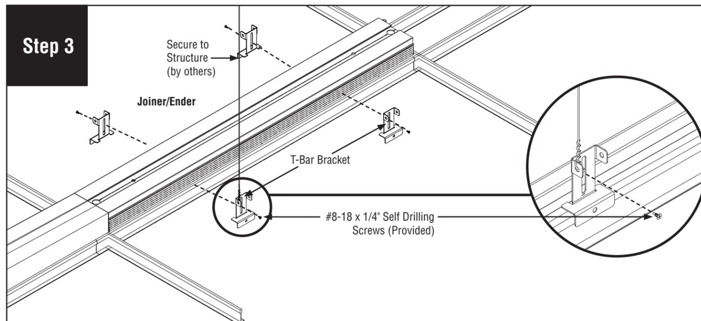
Install T-Bar brackets onto Joiner/ Ender luminaire. Secure with #8-18 x 1/4" screws (provided). Secure luminaire to structure using tie-wire (by others), as per code.
