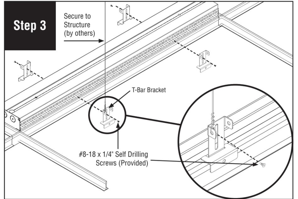
Install T-Bar bracket onto luminaire. Secure with #8-18 x 1/4" screws (provided). Secure luminaire to structure using tie-wire (by others), as per code.
