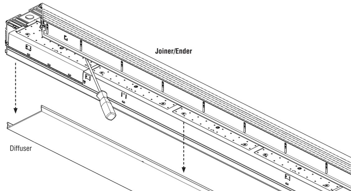
Remove diffuser from Joiner/Ender and set aside to prevent it from getting dirty or damaged. **NOTE:** If part of a longer run, diffuser will be reinstalled back into original luminaire section as lengths vary.
