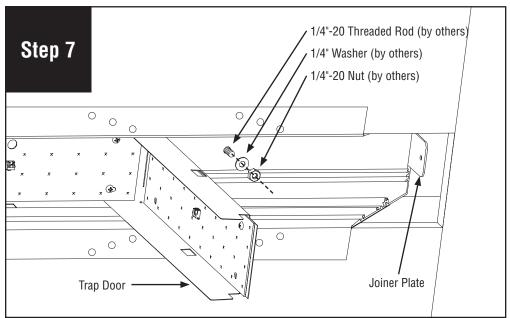
On opposite end of spackle flange luminaire, install 1/4"-20 nut (by others) and 1/4" washer (by others) onto 1/4"-20 threaded rod (by others) or use alternate mounting option (use fastener and washer compatible to structural blocking to secure luminaire).
