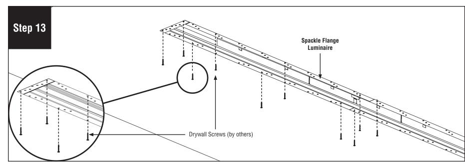
Fasten spackle flange luminaire to the ceiling with drywall screws (by others) through flange into blocking.
