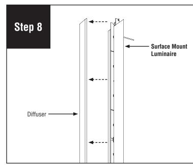
Remove diffuser from surface mount and set aside to prevent it from getting dirty or damaged.
