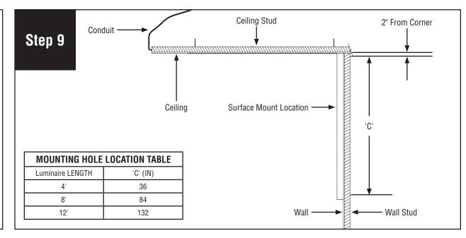
Indicate where surface mount luminaire will be installed. Ensure proper backing (by others).
