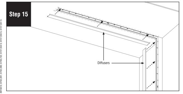
Once the spackling is complete, remove the mud guards, reinstall diffusers, and turn power on to the luminaires. **NOTE:** If part of a longer run, diffuser will be reinstalled back into original luminaire section as lengths vary.
