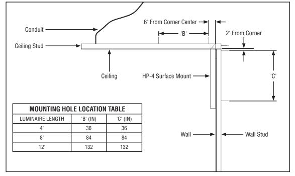
For recessed spackle flange rough in, add 3/4" to the body/row length (A), +/- 1/16" to simplify installation. Luminaire needs to be installed next to support blocking. Use mounting hole location table for mounting positions.
