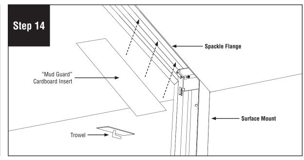
Install the "mud guards" cardboard inserts (provided) to help prevent spackle from getting into the luminaire. Use spackle to cover up the flange before reinstalling the diffuser.
