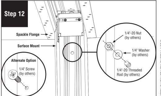
Install 1/4"-20 nut (by others) and 1/4" washer (by others) onto 1/4"-20 threaded rod (by others) or use alternate mounting option. Replace spackle flange and surface mount trap doors and fasten with #8-18 x 1/4" screws (provided).
