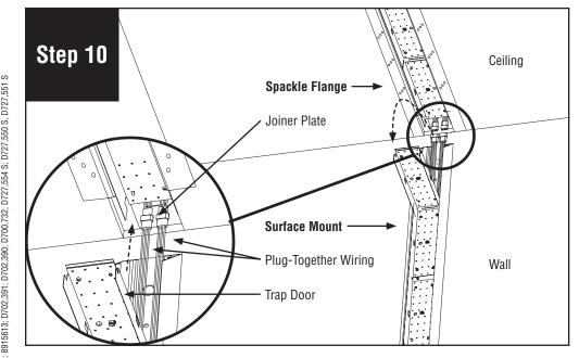
Remove #8-18 x 1/4" screw (provided) to open trap door at both ends of the surface mount. Connect plug-together wiring and slide luminaires together. Align joiner plate with top channel of luminaire.
