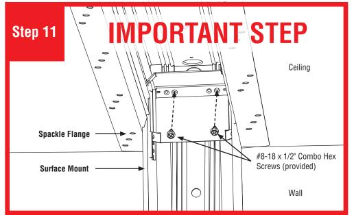
**IMPORTANT STEP:** Install  $2 \#8-18 \times 1/2$ " combo hex screws (provided) into end brackets as shown. Screws can be installed from the left or right. **CAUTION: Do not over-tighten.**
