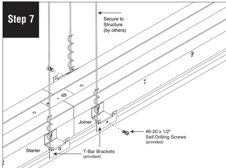
Secure luminaire to T-Bar by driving #6-20 x 1/2" self drilling screws (provided) through the T-Bar brackets (provided) into the T-Bar.
