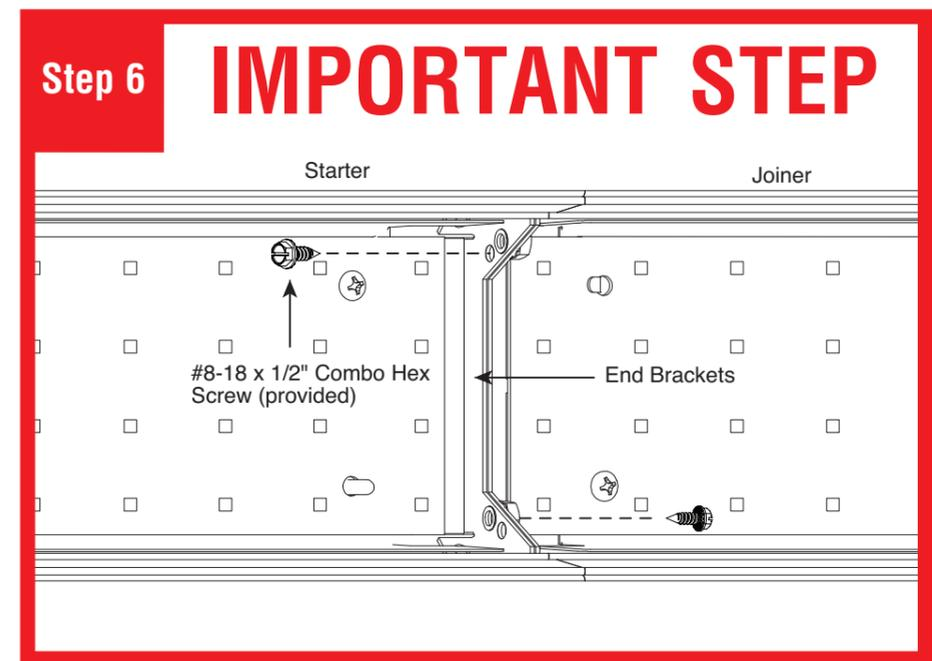
**IMPORTANT STEP:** Install the two #8-18 x 1/2" combo hex screws (provided) into end bracket as shown. Screws can be installed from the left or right. When installed correctly these hex screws will pull luminaires together to make a tight joint.
