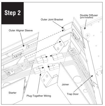
Connect plug-together wiring. Align joint brackets to channels and slide luminaires together.
