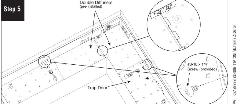
Replace trap doors and fasten with #8-18 x 1/4" screws (provided). Ensure right (long section) diffuser is under left (short section) diffuser tabs.
