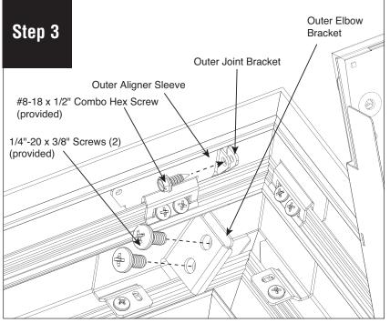
Fasten the outer elbow bracket and aligner sleeve using two 1/4"-20 screws. Then fasten the outer joint bracket and aligner sleeve using one #8-18 x1/2" combo hex screw.
