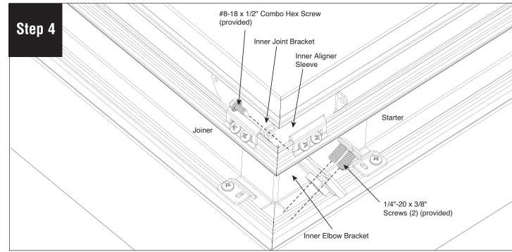
Fasten the inner elbow bracket and aligner sleeve using two 1/4"-20 screws (provided). Then fasten the inner joint bracket and aligner sleeve using one #8-18 x 1/2" combo hex screw (provided).
