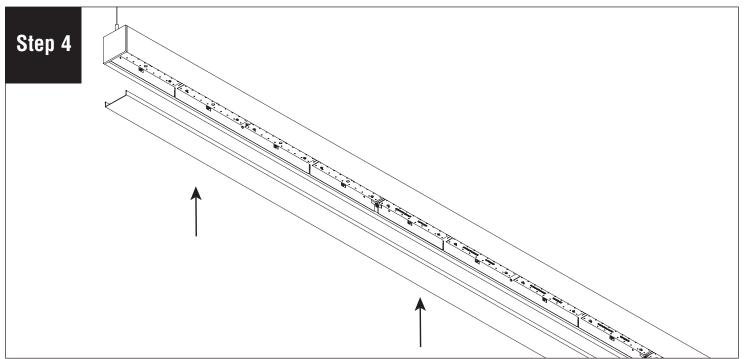
Reinstall lens and turn power on.
