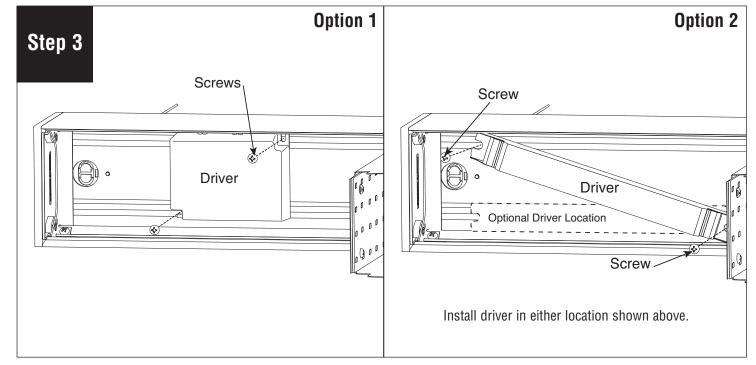
Disconnect all electrical connections from driver(s). Remove mounting screws to replace the new driver. Reconnect all electrical connections and replace trap doors and fasten with #8 screws.
