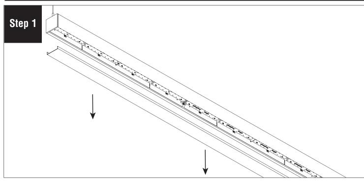
Turn off power. Remove bottom lens and set aside to prevent it from getting dirty or damaged.
