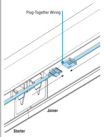
• Connect plug-together wiring.
