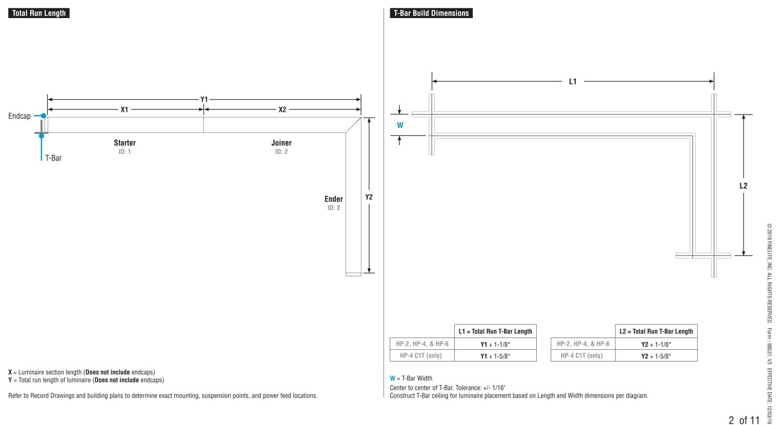
Refer to Record Drawings and building plans to determine exact mounting, suspension points, and power feed locations.
