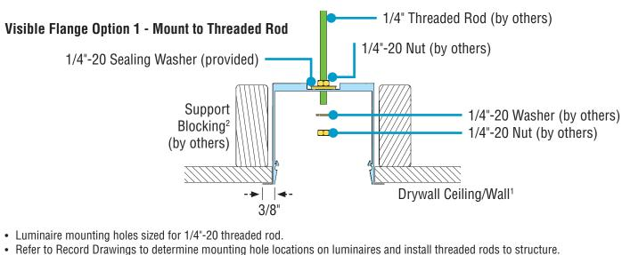
• Distance from threaded rod to wall/ceiling surface<sup>1</sup> must be a minimum of 3-1/2".
