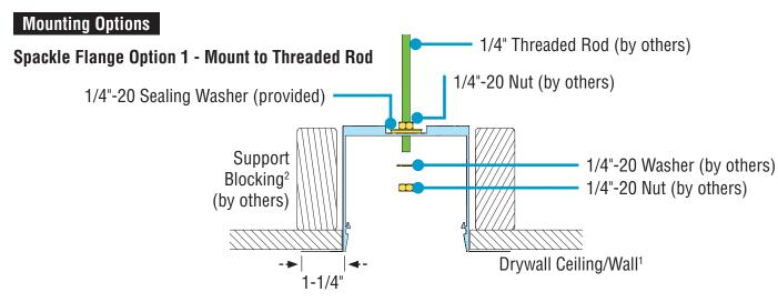
Luminaire mounting holes sized for 1/4"-20 threaded rod.
