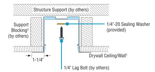
Refer to Record Drawings to determine mounting hole locations on luminaires and install support blocking<sup>2</sup> to structure.
