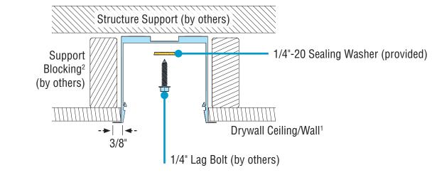
Refer to Record Drawings to determine mounting hole locations on luminaires and install support blocking<sup>2</sup> to structure. • Distance from support block to wall/ceiling surface<sup>1</sup> must be a minimum of 4-1/8".
