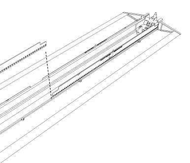
• Replace with new LED engine by peel off wax backing from double sided tape locate on the back of the LED engine.
