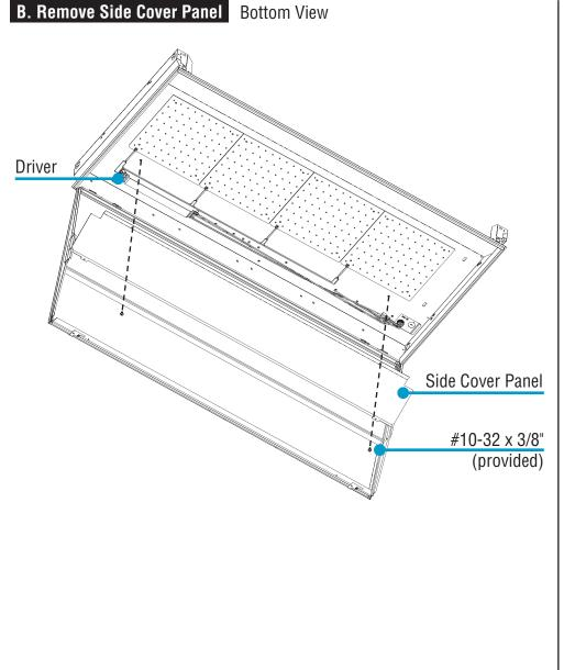
Remove (2) #10-32 x 3/8" screws from side cover panel.
