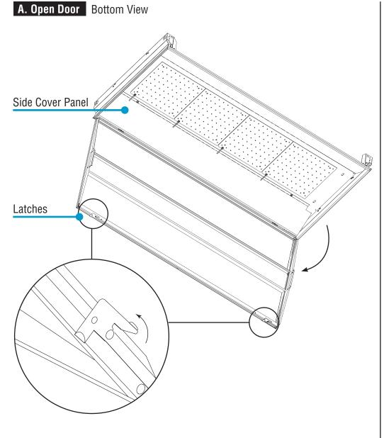
Same procedure for both HPR LED and HPR LED-EP. Disconnect power. Unlock the latches and rotate door to open.
