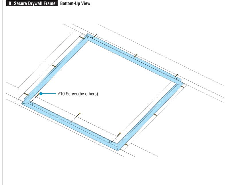
· Fit drywall frame to backing into rough-in opening.
