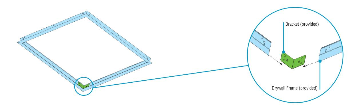
• Slide drywall frame pieces onto brackets until they lock into place.
