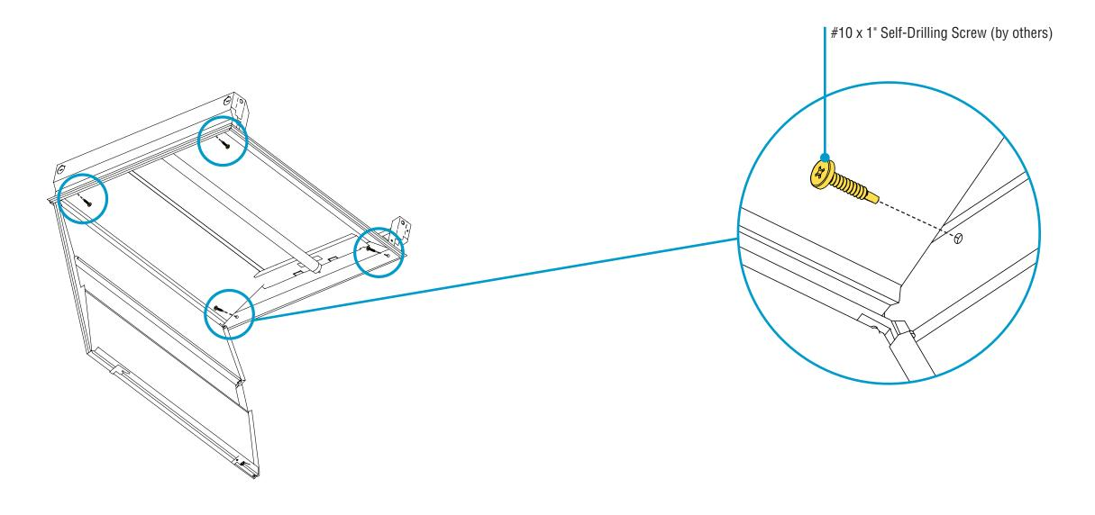
• Once luminaire is installed, secure luminaire to the drywall frame kit using four #10 x 1" self-drilling screws.
