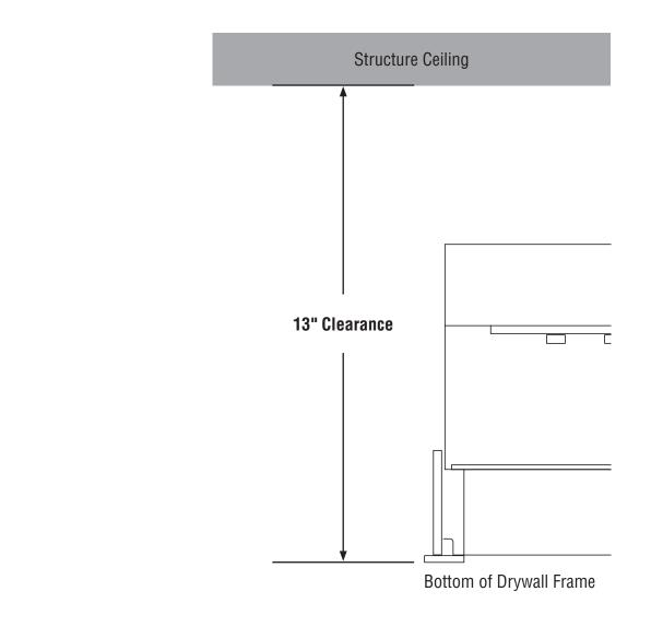
• Minimum height is 13" from bottom of drywall frame to structure ceiling.
