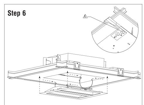
Connect to power according to NEC and other local codes. Install the door by pressing retention springs to align with the cutout on the body. Than press the door into place. If there are light leaks or gaps, please go back to Step 5 to adjust the housing.
