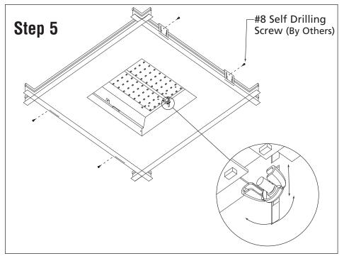
Make sure bottom of the fixture is flush with ceiling. Adjust by using the wing nuts if necessary. Secure the T-Bar brackets to the T-Bar grid by using self drilling screws (by others).
