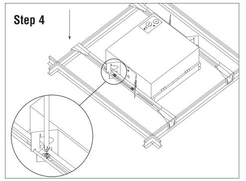
Align the fixture with the cutout on the tile and snap the T-Bar brackets on to the T-Bar grid. Tighten the (4) butterfly bracket screws to the bar hanger.
