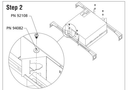
Attach the T-Bar brackets Erico<sup>™</sup> Caddy 512 (supplied by others) to the butterfly brackets as shown. Use screw PN92108 and washer PN94082 (By Finelite). DO NOT TIGHTEN YET.
