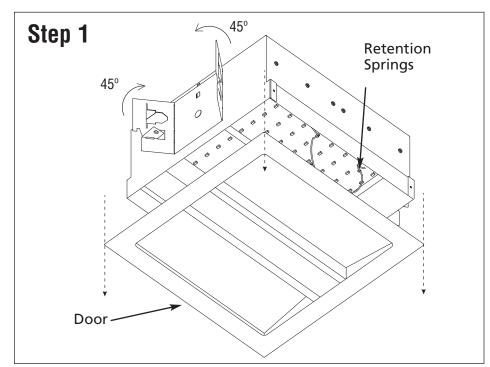
Remove the door by pulling straight down and then squeeze the retention springs until the door is released. Then bend the butterfly brackets about 45° on both sides.
