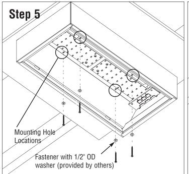
Install fixture using appropriate fastener with 1/2" OD washer (provided by others) at mounting hole locations.
