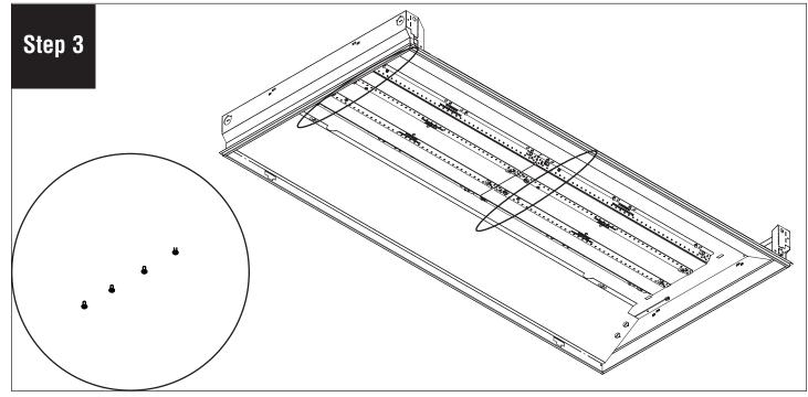
Remove all screws holding the LED boards.
