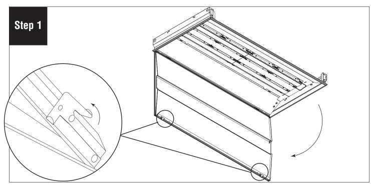
Disconnect power. Unlock the latches and rotate door to open.
