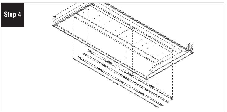
Remove old LED boards and replace with new boards. Secure new boards using #6-32 x 3/16 screws (provided). Reconnect all jumpers and close luminaire door. Turn power on to fixture.
