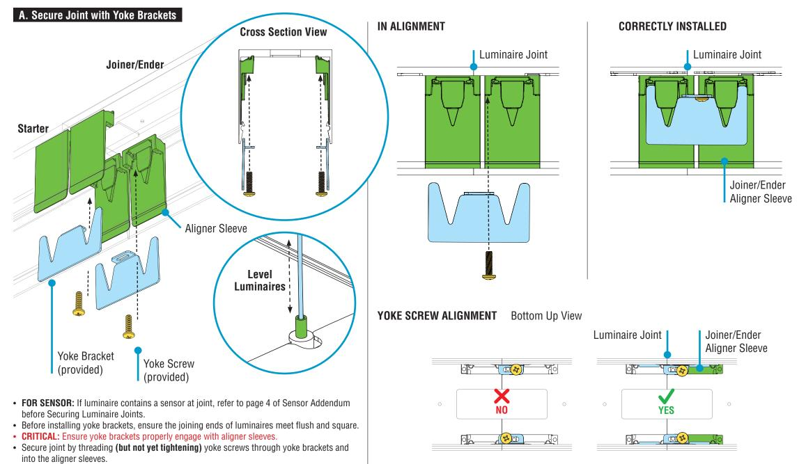
• Level all luminaires to desired height by depressing top of grippers to adjust cable lengths.
