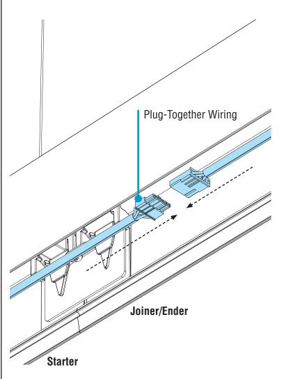
• Connect plug-together wiring.
