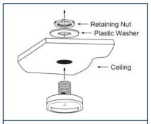
Standard drop ceiling mounting. Cut a 13/16" hole in the ceiling tile where the daylight sensor is to be mounted.
