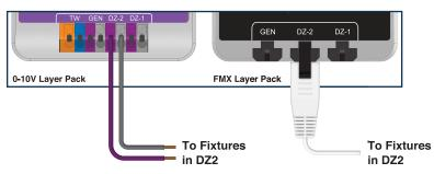
Daisy chain connections to all fixtures falling within Daylight Zone 2.
