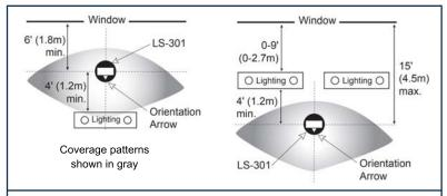
Placement for applications where lighting fixtures are outside of 10 feet of davlight source.
