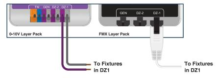
• Daisy chain connections to all fixtures falling within Daylight Zone 1. All fixtures connected will dim according to the amount of daylight the Daylight Sensor connected to DZ1 is measuring.
