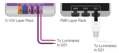
Daisy chain connections to all luminaries falling within Daylight Zone 1.
