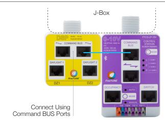
Connect the Daylight Sensor Pack to a Layer Pack using CAT5 to provide power and allow for Daylight Sensor data to pass through to all connected devices.
