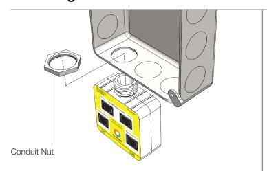
Place the Daylight Sensor Pack through a 34" knockout and securely fasten conduit nut.
