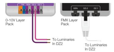
Daisy chain connections to all luminaries falling within Daylight Zone 2.
