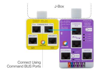
Connect the Daylight Sensor Pack to a Layer Pack using CAT5 to provide power and allow for Daylight Sensor data to pass through to all connected devices.
