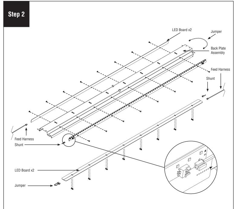
Remove #10 screws (2) from both ends of back plate assembly, then remove the back plate assembly. Remove diffusers (2) from back plate assembly.
