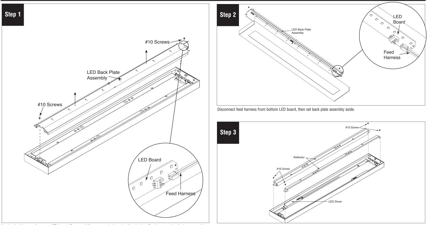
Unplug feed harness from top LED board. Remove #10 screws on both ends of back plate. Gently remove back plate assembly.
