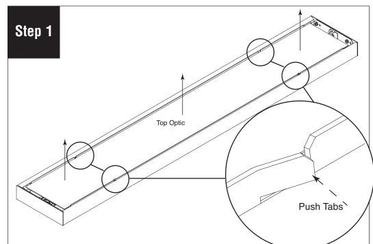
Remove top optic by pushing in the tabs. If top optic is not used, go to step 2.
