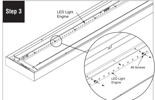
Remove (8) #6 screws that holding the LED light engine to the reflector and remove light engines on both sides. Reverse steps to install the new LED light engine.
