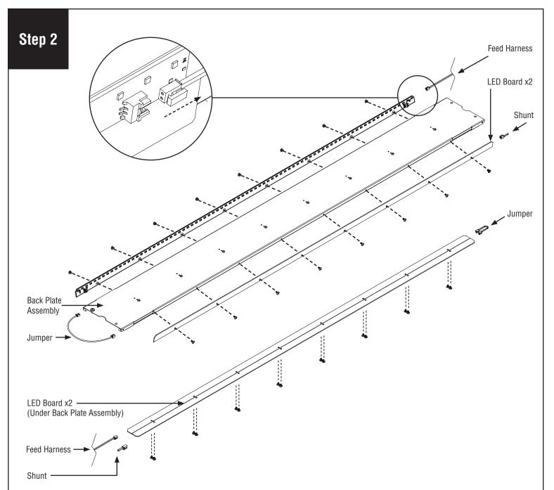
Remove #10 screws (4) on both ends of back plate assembly, then remove the back plate assembly.
