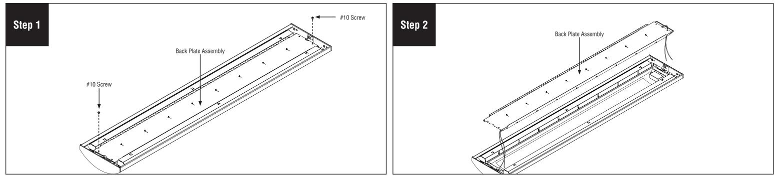
Remove #10 screws (2) from both ends of back plate assembly, then remove back plate assembly.
