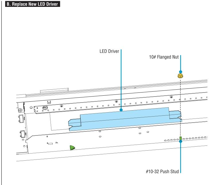
• Remove #10 flanged nut that secures the LED driver(s) and replace with new driver(s). Reverse steps to reassemble luminaire.
