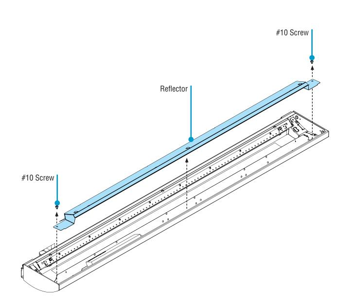
• Remove #10 screws from both ends of the reflector. Remove reflectors to access LED driver(s). Disconnect all feed harnesses.
