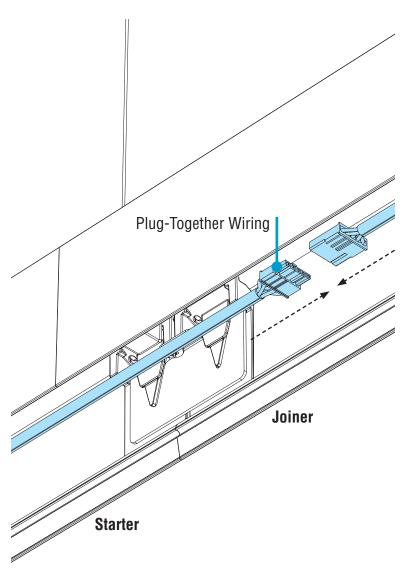
Connect plug-together wiring.
