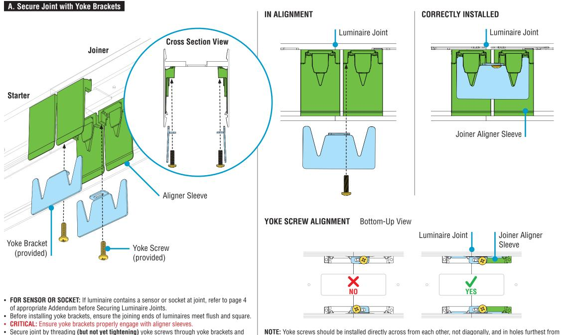
• Secure joint by threading (but not yet tightening) yoke screws through yoke brackets and into the aligner sleeves.
