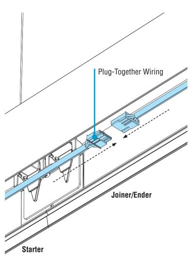
• Connect plug-together wiring.
