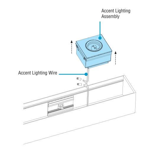
• Once backplates are open, release accent lighting assembly by gently sliding the blade of a putty knife between accent lighting assembly and luminaire body.
