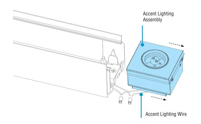
· Once backplates are open, remove tape holding accent lighting assembly onto luminaire and discard.
