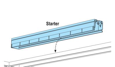
• Lower starter luminaire into place onto T-Bar.
