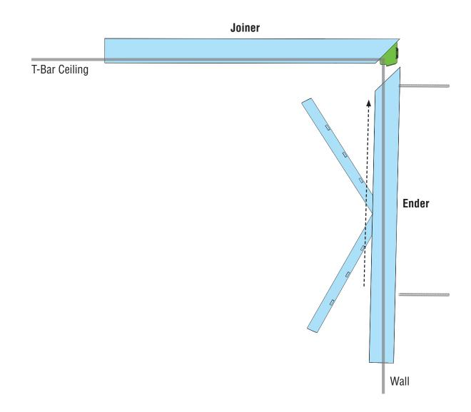
· With all backplates open, carefully maneuver ender luminaire to wall opening and insert at an angle.
