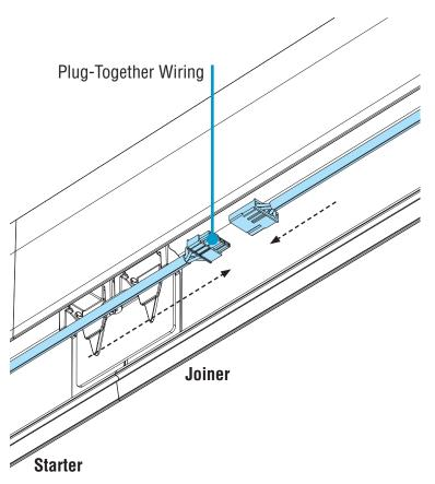
• Connect plug-together wiring.
