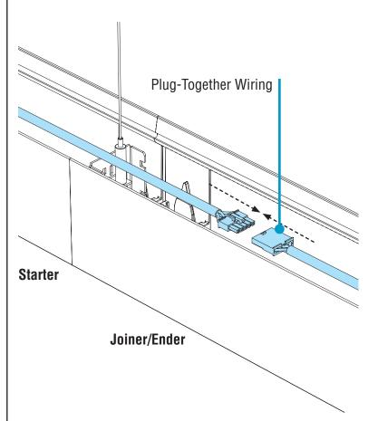
• Connect plug-together wiring.
