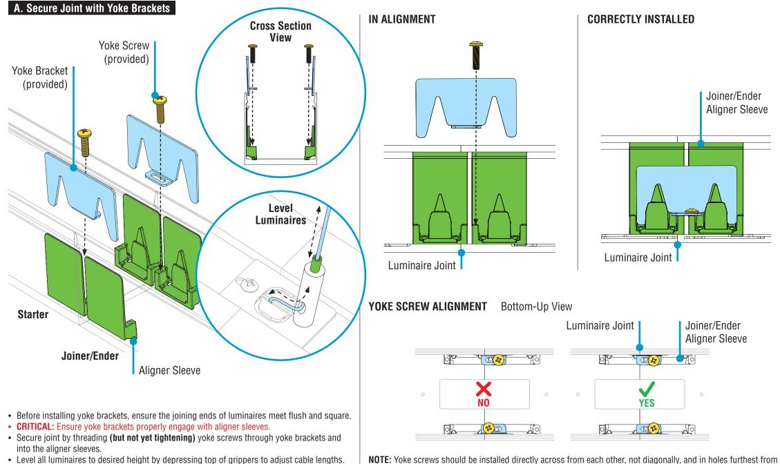
the joint line. One voke screw per one voke bracket.
