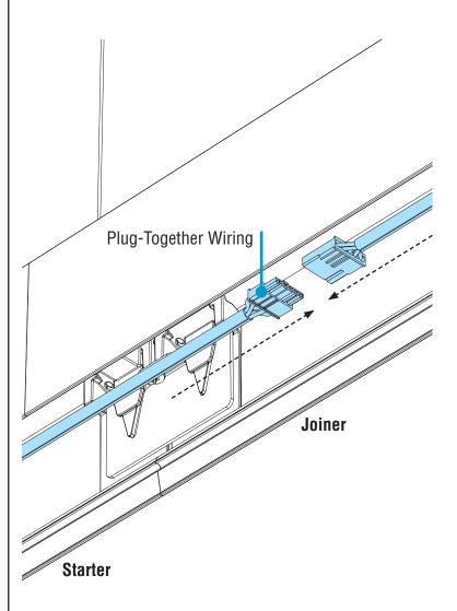
Connect plug-together wiring.
