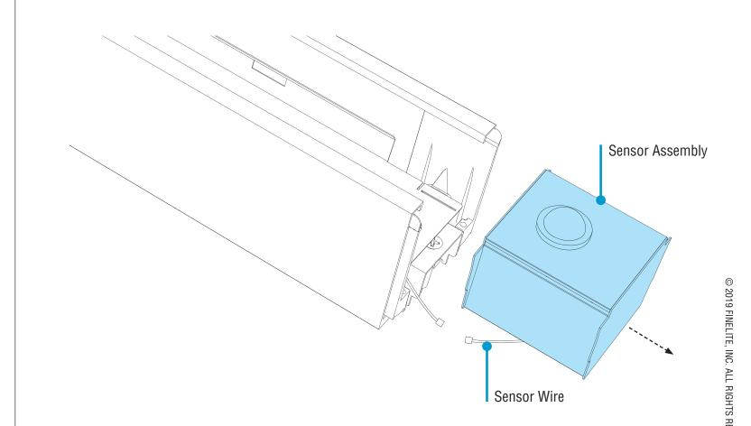
• Remove tape holding sensor assembly onto luminaire and discard.
