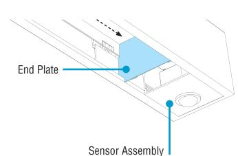
• Once luminaire is mounted and backplate is replaced, reconnect sensor wire to sensor assembly.
