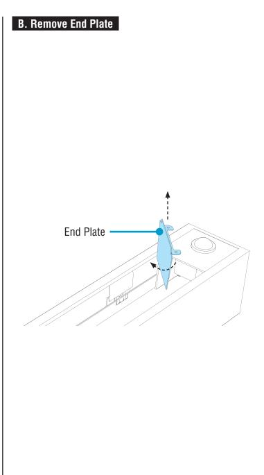
· Rotate end plate and remove from luminaire.
