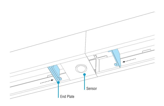
• Rotate end plates and insert into luminaire.
