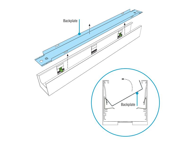
• Use putty knife to slip behind backplate edges and release backplate from clips.
