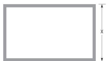
Measurements are made to the outside of the luminous area as shown above for configurations. Minimum length of any section (X) is 4'.
