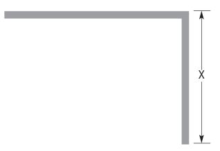
Measurements are made to the outside of the luminous area as shown above for single corner. Minimum length of any section (X) is 2'.
