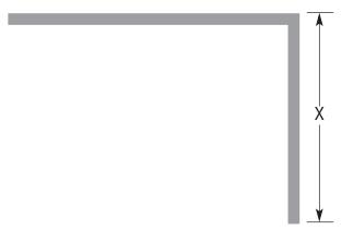
Measurements are made to the outside of the luminous area as shown above for single corner. Minimum length of any section (X) is 2'.
