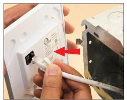
Connect Cat5 cable to the back of the wall controller.
