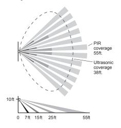
Coverages shown are maximum and represent half-step walking motion. Under ideal conditions with no barriers or obstacles, coverage for half-step walking motion can reach up to 2000 ft², while coverage for typical desktop activity can reach up to 1000 ft².
