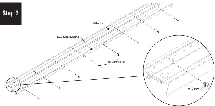
Remove (8) #6 screws that hold the LED light engine to the reflector and remove light engines on both sides. Reverse steps to install the new LED light engine.
