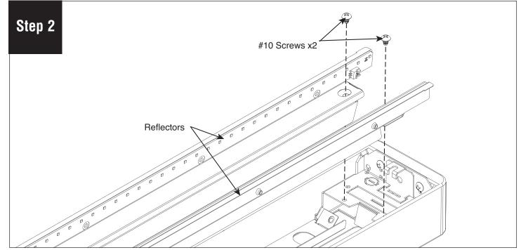
Remove (4) #10 screws that hold the reflectors into the fixture, take reflectors with the LED light engines out of the fixture.
