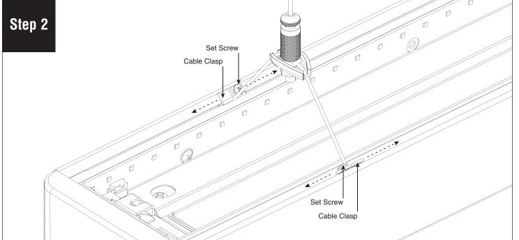
Slide the cable clasps to desired position while keeping tension. Maximum distance from endcap: 1' on 4' body sections, 2' on 8' body sections. Retighten the set screws.
