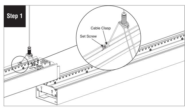
To adjust the position of the mounting point, use a Philip's head screwdriver to loosen cable clasp set screws without removing them. Max distances of flexible mount location from end of body 1' for 4' body, 2' for 8' body.
