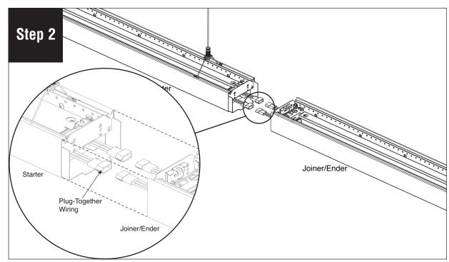
Connect plug together wiring, then slide the luminaires together. Be careful not to damage wiring.
