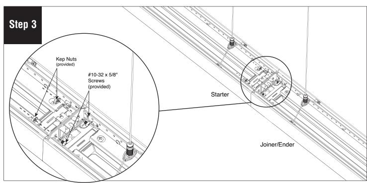
Secure joint with #10-32  $\times$  5/8" screws (provided) and tighten kep nuts (provided). Level luminaire then turn power on.
