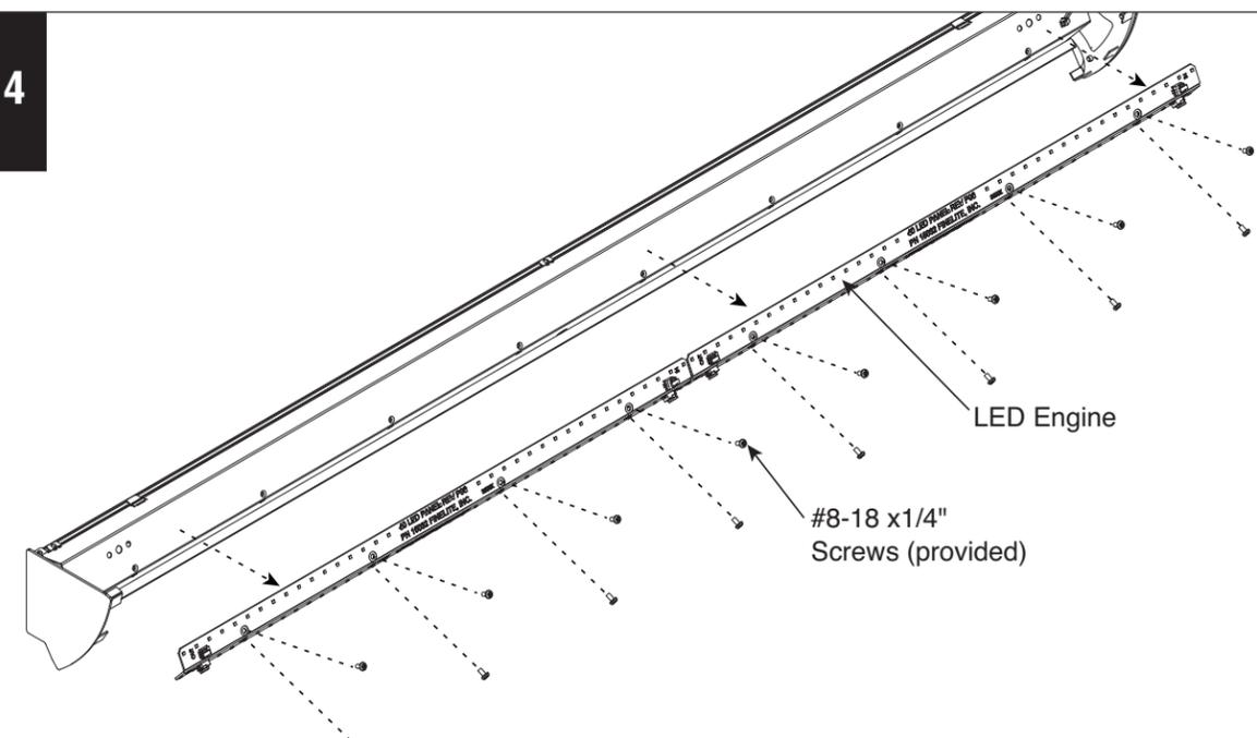
Remove #8-18 x 1/4" screws (provided) and old LED boards. Install new LED boards using same screws. Replace lenses and fascia. Turn power on to fixture.
