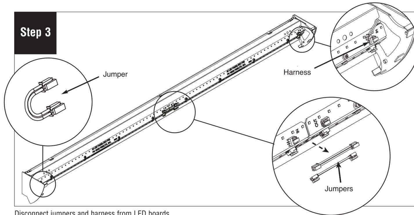
Disconnect jumpers and harness from LED boards.
