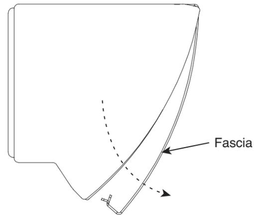
Remove fascia from fixture by pulling outwards.
