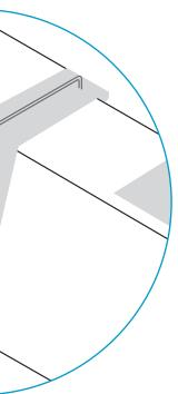
Chicago Plenum Tape (Provided) Note: Tape is not transparent. Holes shown to illustrate what to cover up.
