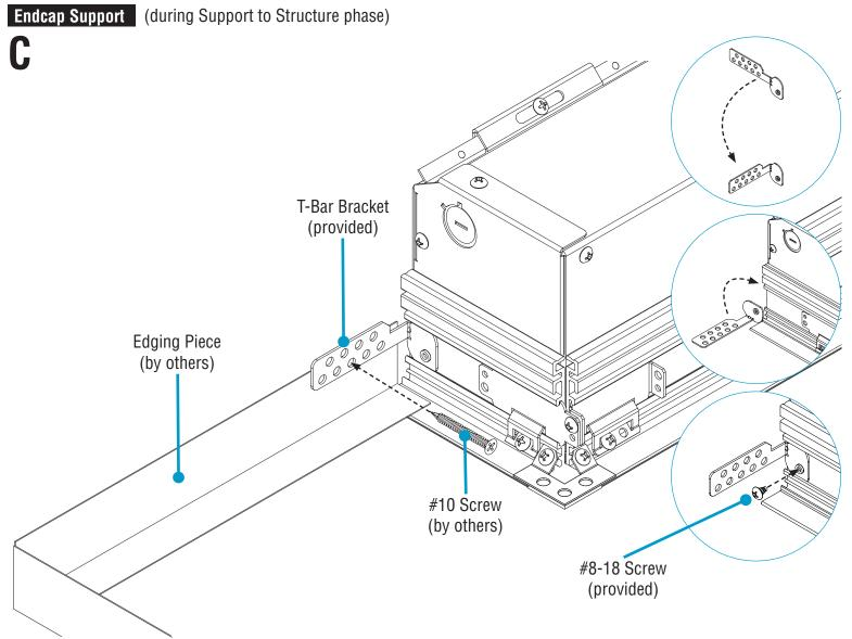
Locate a T-Bar Bracket (provided). Bend it 90 degrees as shown. Align the T-Bar Bracket to the slot in the extruded portion of the Pocket Endcap. Rotate the T-Bar Bracket 90 degrees so the tab with holes is parallel to the wall. Put in edging piece. Slide T-Bar Bracket towards the wall until contact. Set bracket into place by screwing in a #8-18 screw (provided). Use appropriate #10 screws (by others) to fasten T-Bar Bracket to wall.
