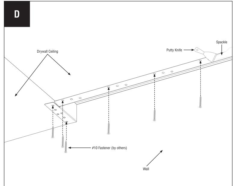
The end cap has a Spackle Flange similar to what runs the length of the fixture. Provide support blocking to attach the drywall through the Spackle Flange End Cap and secure the fixture to the wall.
