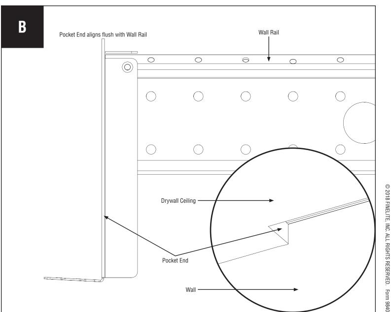
For Wall Rail placement, use the table to help you find where the height of the Wall Rail will be mounted. Mark wall for "Y" dimension, make sure lines are level.
