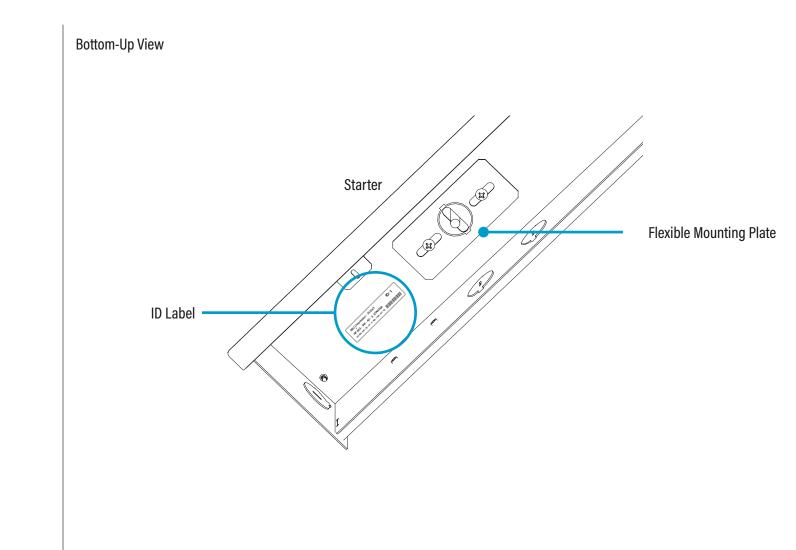
· Identify all luminaires by their ID label that can be found on the box and inside the luminaire.
