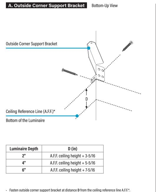
Fasten bracket using appropriate #10 screws.
